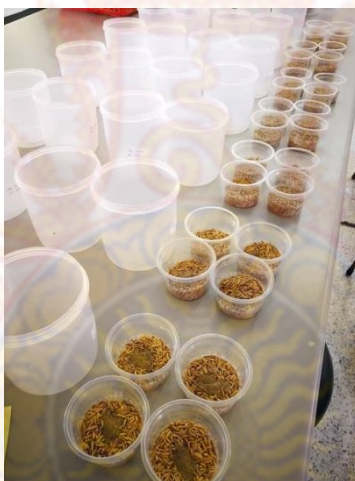
Figure 3.11 Repellent activity test of powders of tested plants against adults of S. oryzae or R. domonica by cup bioassay method
