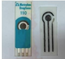
Figure 4. Photograph comparing DropSens 110 and homemade SPCE.
